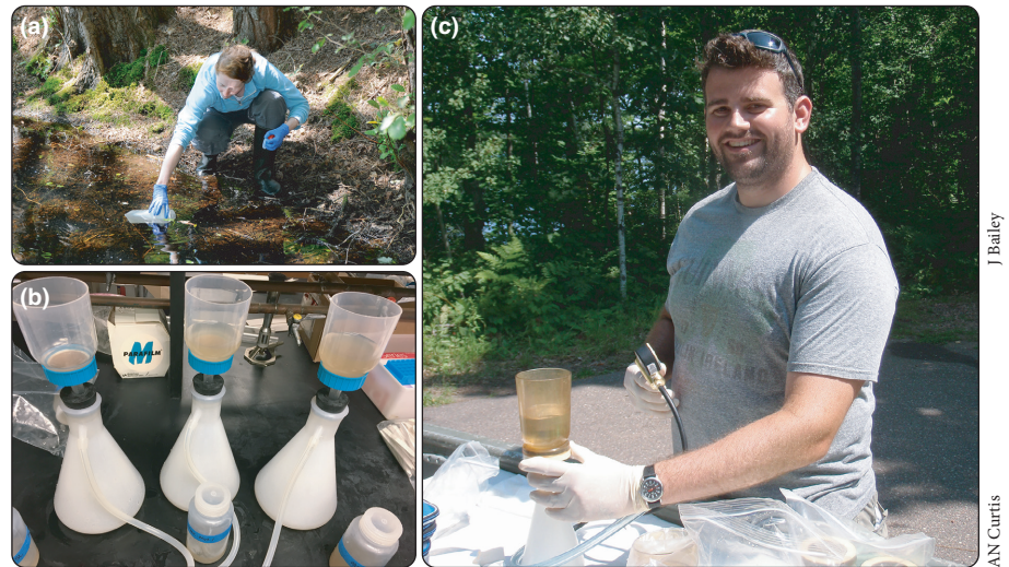
Figure 1. A typical process of using eDNA for invasive species surveillance includes (a) collecting environmental samples and (b) capturing DNA through a method like filtering water through fine pore cellulose nitrate filters, which may be performed in the laboratory or (c) immediately under field conditions. Stored samples can then be extracted in the laboratory and analyzed using single species (eg quantitative or real-time PCR) or multispecies (eg metabarcoding) approaches.
