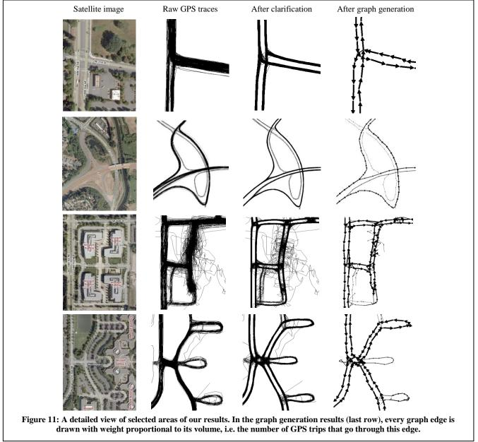
generation algorithm to generate a directed graph describing the connectivity and geometry of the road network. We then show that the resulting graph is able to answer route planning queries satisfactorily.
