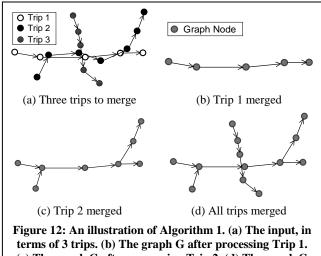
terms of 3 trips. (b) The graph G after processing Trip 1. (c) The graph G after processing Trip 2. (d) The graph G after processing Trip 3.
