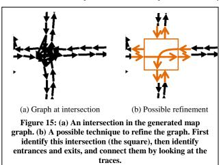
"entrances" and "exits" of this intersection. Finally, we connect "entrances" to "exits" by looking at the traces – if there is a trace that enters from an "entrance" and exits from an "exit", we connect the "entrance" and the "exit".
