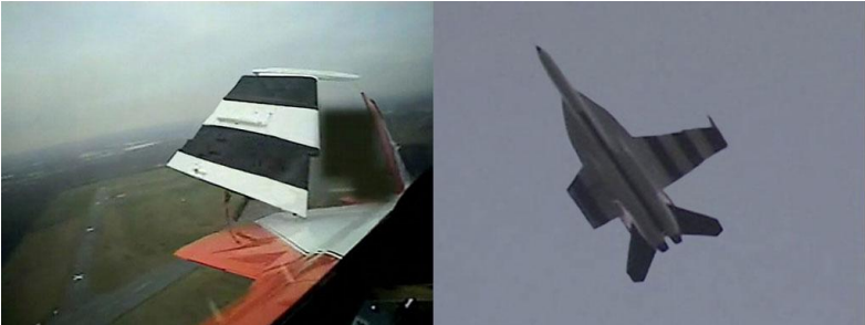
Successful flight demonstration of damage tolerant flight control and autonomous landing capabilities on an unmanned sub-scale F/A-18 on April 18, 2007 in Maryland.
