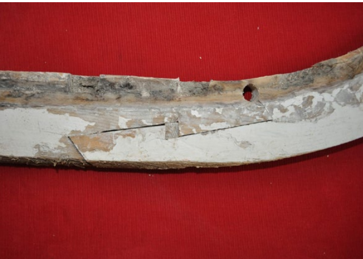
A scarp joint. Courtesy The Wooden Boat Museum of Newfoundland and Labrador.
