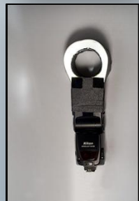
(Figure 7 - Home made macro ring flash adaptor.)
