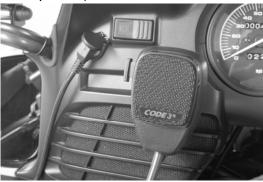
The BMW / Code 3 siren is a 100W system featuring wail, yelp, hyper-yelp and air horn tones, as well as radio rebroadcast and public address when connected. The system is California Title 13 certified with the Code 3 speaker and Federal Signal Dynamax MS100 speaker.
