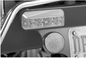
Emergency lights are powered by the auxiliary battery and function with the ignition "on" or "off". The strobe emergency lights operate using the emergency light switch. Rock the switch down to activate the strobe lights. The middle position activates the rear strobe lights (amber dashboard LED) and the lower position activates all strobe lights (red dashboard LED).
