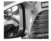
**Note:** Earlier production motors have a rocker RRB switch (trumpet emblem) beside the heated grip switch. Rock that switch down for RRB, middle and upper positions are "off".
