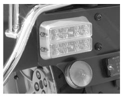
Emergency lights are powered by the auxiliary battery and function with the ignition "on" or "off". The strobe emergency lights operate using the emergency light switch. Rock the switch down to activate the strobe lights. The middle position activates the rear strobe lights (amber dashboard LED) and the lower position activates all strobe lights (red dashboard LED).
