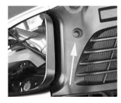
**e. Heated Handlebar Grips:** This rocker switch activates the standard heated grips. Rock down for low heat, rock all the way up for high heat, "off" in the middle position. This location differs from the location noted in the Rider's Manual, as the original factory heated grip switch is used for the emergency lights.
