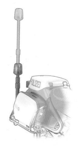
The telescoping strobe pole light operates when the rear emergency lights are activated and when the beacon switch is pressed down. The telescoping strobe pole light can be operated in the fully lowered position (providing 270 degree illumination) while the motorcycle is being driven, or extended when the motorcycle is parked to provide 360 degree illumination. Extending both pole sections can elevate the telescoping strobe light up to 6 ½ feet above the road surface.
