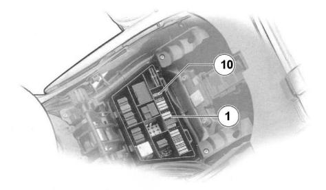
A secondary block of fuses, located under the seat beside the normal civil fuses, is provided for emergency equipment. Most of these fuse circuits obtain power from the auxiliary battery, thereby reducing the likelihood that the main motorcycle battery will be discharged and unable to restart the motor or pass ABS self-test.
