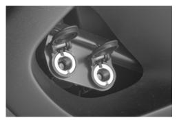
A charging outlet is provided to enable officers to charge batteries during periods of storage. The forward outlet charges the auxiliary battery and the rearward outlet charges the main motor battery. Note that each battery must be charged separately – charging one does not automatically charge the other.
