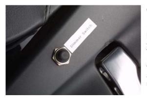
On models equipped with the Whelen UPS690 strobe amplifier, a dimming switch is provided. With the emergency lights "on", pressing this button will dim the strobe amplifier output to reduce the intensity of the strobe lights. This function is often used in foggy conditions. To regain full intensity, turn the emergency lights "off", then "on" again. Cycling the lights "off" will reset the strobe amplifier to full intensity.
