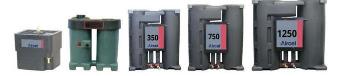
Compressor condensate typically contains as much as 5% oil, making it too harmful to the environment to be discharged without purification. Condensate drain valves reliably discharge compressed air condensate from the pressurized system. Oil/water separators process condensate to a residual oil content as low as 10 ppm, allowing the processed water to be discharged into most municipal waste water treatment systems.
