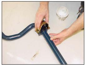
6/ Lift the bar up to the vehicle with the two smaller H-Sport stickers at the ends right-side-up. As you lift the bar up to the mounting points, <u>you must</u> place one mounting plate per side between the bushing and the mounting point. This relocates the bushing out of the stock bushing pocket. Re-install the bracket nuts and tighten. <u>Re-install the end link bolts and tighten well using medium strength thread locker</u>.
