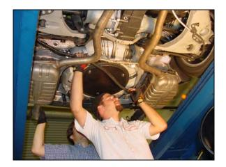
7/ Repeat same pressure to the exhaust and position H-Sport bar (without the bushings and brackets) in the stock location with the "H-Sport" sticker facing rearward, right side up.
