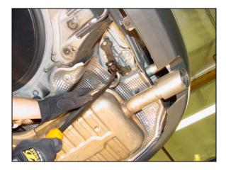
4/ Remove the two lower end link bolts (16mm wrench) which attach the sway bar ends to the end links. You may need to hold the wrench-flat with a 17mm wrench.
