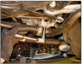
5/ Apply second tube of grease to each inner-channeled portion of the two new front bushings and attach to H-Sport bar against the outside of the washers. Slip the new brackets over the bushings.
