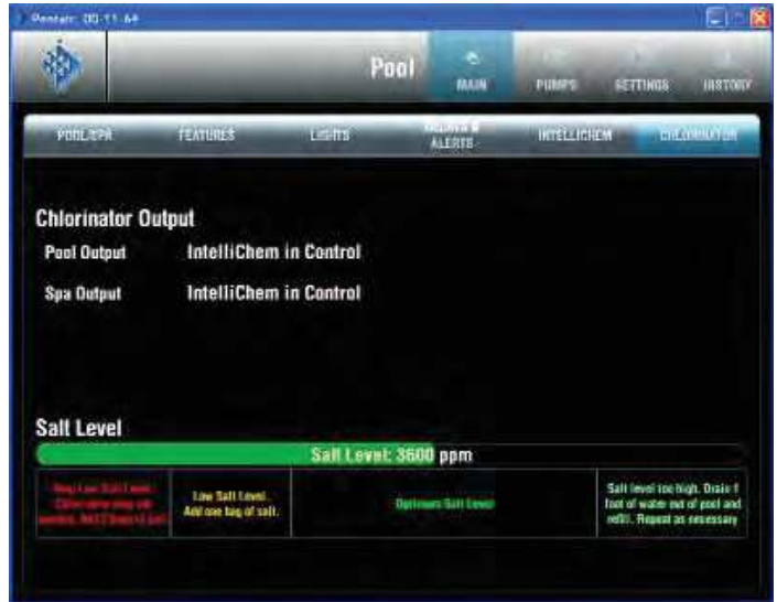
Chlorinator (IntelliChlor) with IntelliChem controller screen
