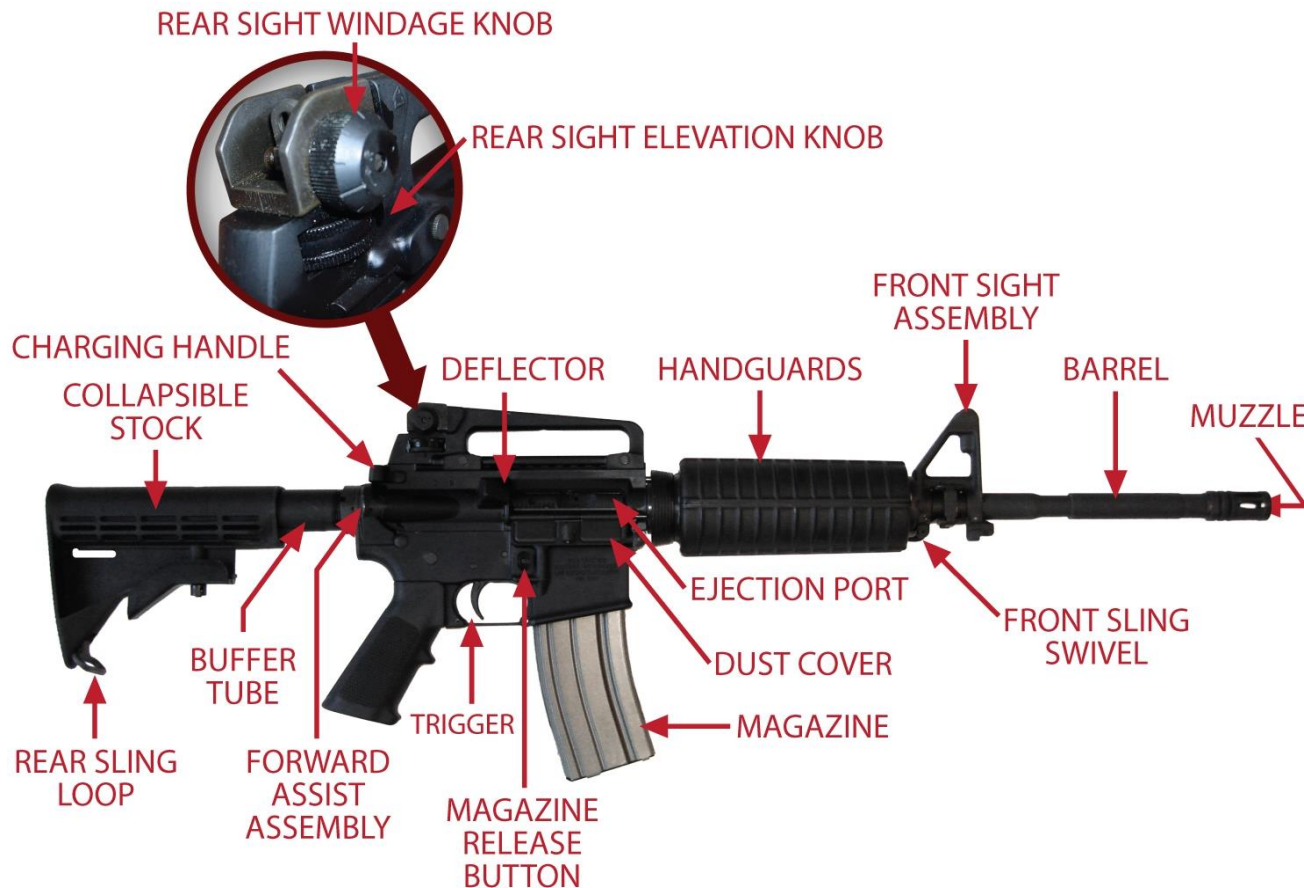
Figure 20. AR-15 Rifle Nomenclature and Controls, Right Side
