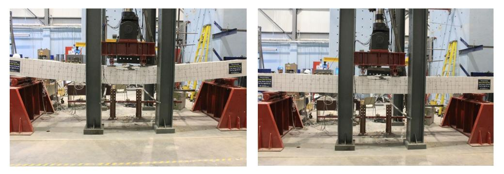
When the applied load was released, the FRP RC beam recovered most of their deflection during the unloading process, because the FRP bars on the tension side did not reach rupture strain; In contrast, the steel specimen retained deflection after unloading (Elastic behavior of FRP: Resilient structural element which maintains its functionality)
