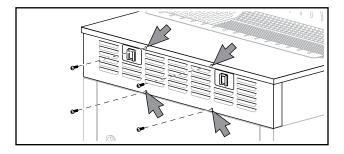
Slide down and tilt out the Front Housing panel away from unit.
