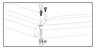
14. Remove and retain the four (4) screws securing the Calrod Heater to the affected Fan Assembly.
