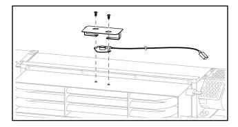
8. Apply heat transfer compound to the mounting surface of the replacement High Limit Thermostat(s).
