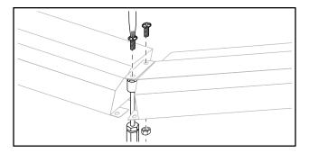
22. Remove and retain the four (4) screws securing the Calrod Heater to the affected Fan Assembly.
