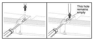
24. Reinstall the bottom front hex nut/bolt. Due to the space between the Heater/Fans, you may need to use a finger to hold up the hex nut while inserting and securing the bolt.
