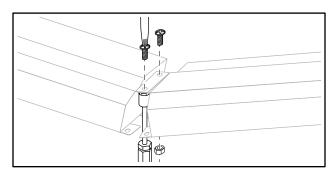
14. Install the replacement Heater/Fan by first reconnecting the two (2) top hex nuts/bolts securing the two (2) Heater/Fans together, with the Heater/Fans at an angle.
