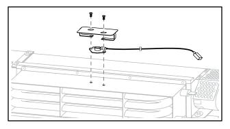
8. Remove and retain the four (4) screws securing the Calrod Heater to the Fan Assembly.
