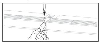
25. Reinstall the reassembled Heater/Fan Assembly and fan guards into the fan base and unit by reversing the previous steps.
