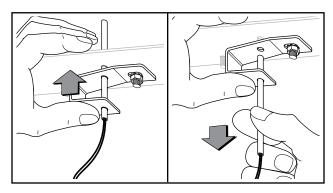
9. Insert the replacement Thermocouple into the bracket. Make sure the Thermocouple extends 1-1/8" (28.6 mm) above the panel.
