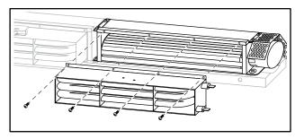
9. Attach the replacement Calrod Heater to the Fan Assembly with its screws.
