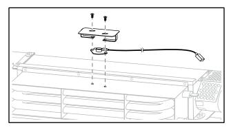
16. Remove and retain the four (4) screws securing the Calrod Heater to the Fan Assembly.
