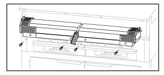
13. Slide the Heater/Fan Assembly with its Fan Base out enough to access electrical connections.
