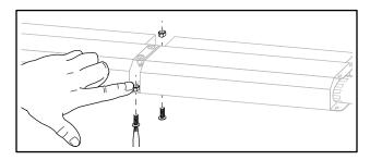
20. With the two top hex nuts/bolts still installed, slightly separate, at an angle, the two Heater/Fans to allow for access to the two hex nuts/screws.
