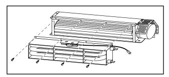
15. Attach the replacement Fan Assembly to the Calrod Heater with its screws.
