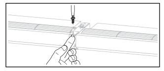
19. Reinstall the reassembled Heater/Fan Assembly and motor guards into the Fan Base and unit by reversing the previous steps.
