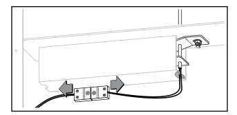
7. Remove and retain the two (2) 3/8" hex nuts securing the Thermocouple switch guard and remove from unit.
