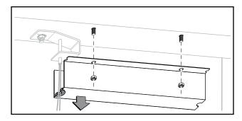
8. Compress the bracket to release the tension and carefully pull out the effected Thermocouple. **NOTE**: it is not necessary to remove the bracket.
