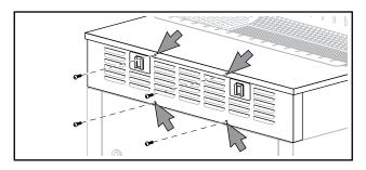
3. Slide down and tilt out the Front Housing away from unit.
