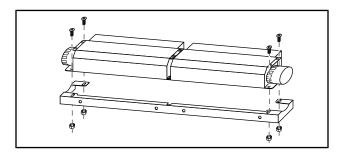
19. Remove and retain the two (2) bottom 11/32" (9mm) hex nuts/bolts holding the two (2) Heater/Fans together. May need to use a finger or screwdriver to assist in holding the hex nut.
