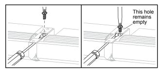
17. Reinstall the rear bottom hex nut/bolt. Due to the space between the Heater/Fans, you may need to use a finger to hold up the hex nut while inserting and securing the bolt.
