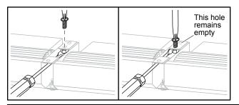
26. Reinstall the front bottom hex nut/bolt. Due to the space between the Heater/Fans, you may need to use a finger to hold up the hex nut while inserting and securing the bolt.
