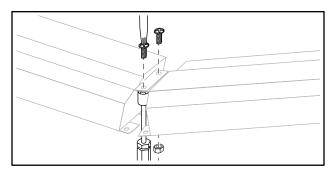
22. Install the replacement Heater/Fan by first reconnecting the two (2) top hex nuts/bolts securing the two Heater/Fans together, with the Heater/Fans at an angle.
