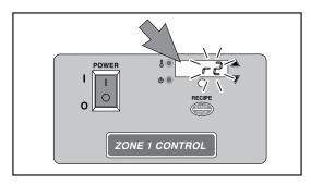
b. The current recipe can be changed by pressing the "Up" or "Down" key.
