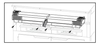
13. Slide the entire Heater/Fan Assembly, with its Fan Base, out enough to access electrical connections.
