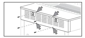
3. Slide down and tilt out the Front Housing away from unit.
