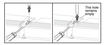
16. Reinstall the front bottom hex nut/bolt. Due to the space between the Heater/Fans, you may need to use a finger to hold up the hex nut while inserting and securing the bolt.
