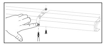
20. With the two (2) top hex nuts/bolts still installed, slightly separate, at an angle, the two Heater/Fans to allow for access to the two hex nuts/screws.
