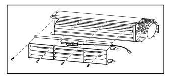
23. Attach the replacement Fan Assembly to the Calrod Heater with its screws.
