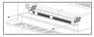
Carefully slide the entire Heater/Fan Assembly out enough to access its electrical connections.
