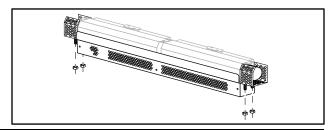
Remove and retain the two (2) bottom 11/32-inch hex nuts/bolts holding the two (2) Heater/Fans together.
