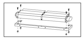
Remove and retain the two (2) bottom 11/32" (9mm) hex nuts/bolts holding the two (2) Heater/Fans together.
