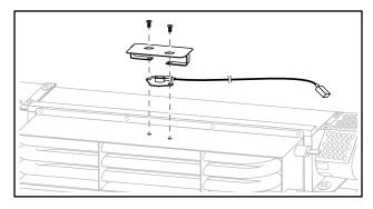
16. Apply heat transfer compound to the mounting surface of the replacement High Limit Thermostat(s).
