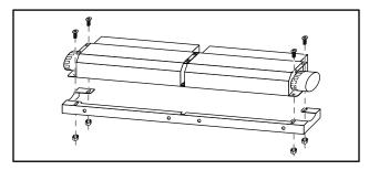
19. Remove and retain the two (2) bottom 11/32" (9mm) hex nuts/bolts holding the two (2) Heater/Fans together. May need to use a finger or screwdriver to assist in holding the hex nut.
