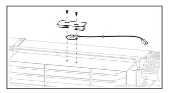
Remove and retain the four (4) screws securing the Heater to the Fan.
