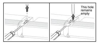
18. Reinstall the front bottom hex nut/bolt. Due to the space between the Heater/Fans, you may need to use a finger to hold up the hex nut while inserting and securing the bolt.
