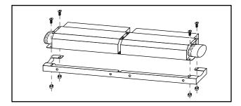
11. Remove and retain the two (2) bottom 11/32" (9mm) hex nuts/bolts holding the two (2) Heater/Fans together. May need to use a finger or screwdriver to assist in holding the hex nut.
