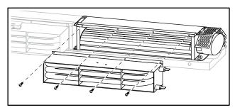
17. Attach the replacement Calrod Heater to the Fan Assembly with its screws.
