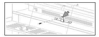
Remove the two (2) screws securing the Fan Bracket to the unit.
