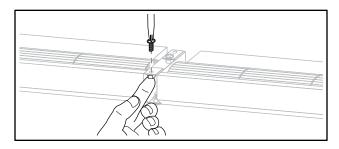
16. Reinstall the front bottom hex nut/bolt. Due to the space between the Heater/Fans, you may need to use a flathead screwdriver to hold up the hex nut while inserting and securing the bolt, then use the screwdriver as a wedge to prevent the hex nut from spinning.
