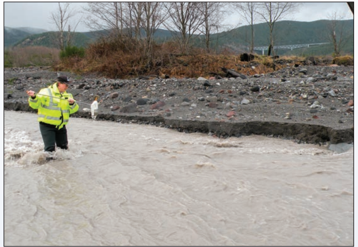
Photograph of Tami Christianson taking a sample from the Toutle River using a handheld suspended-sediment sampler. Photograph taken December 14, 2010, by Emily Roeder, U.S. Geological Survey volunteer.
