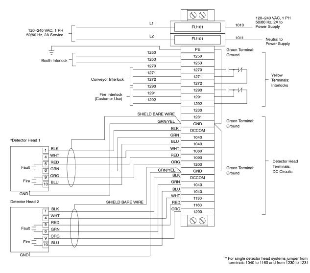
Figure 6 Installation Wiring Diagram – Indicator Panel 307445 without Field Wiring Connectors
