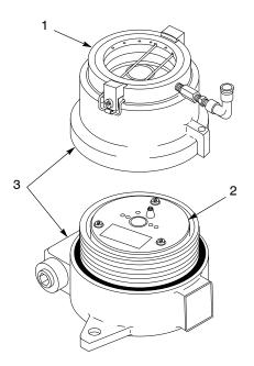
Figure 2 Detector Head Components
