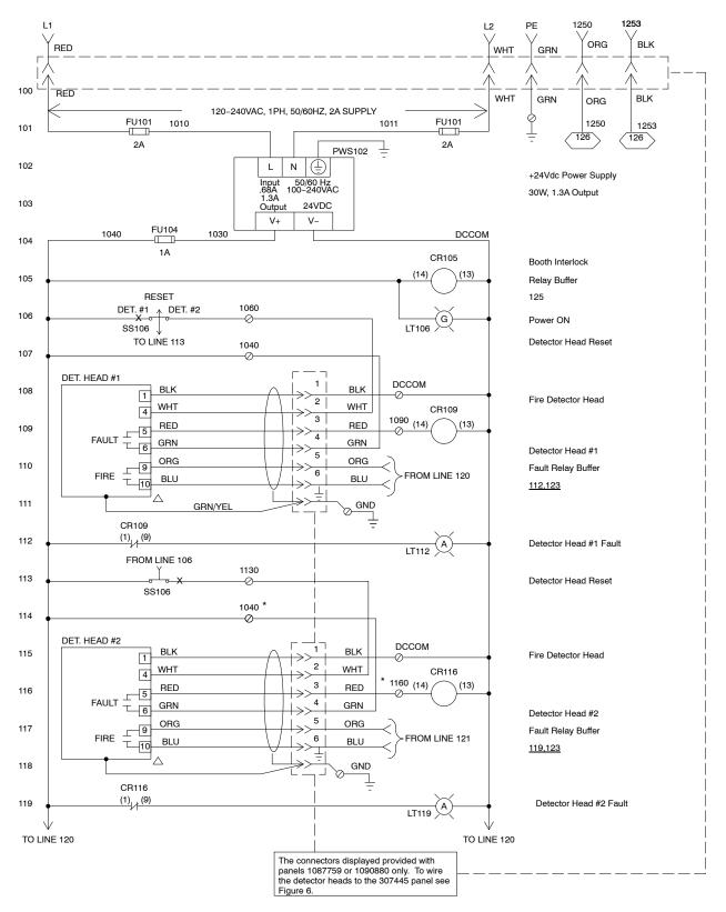
Figure 8 Indicator Panel Electrical Schematic (Sheet 1 of 2)
