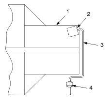
Figure 4 Detector Head Pneumatic Connections
