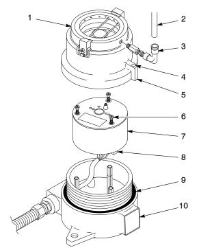
Figure 9 **Detector Head Electrical Connections**
