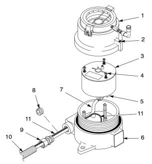
Figure 5 **Detector Head Electrical Connection**
