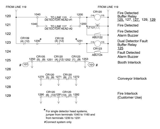
Figure 7 Indicator Panel Electrical Schematic (Sheet 2 of 2)
