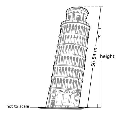
In the 1990s, engineers restored the building so that angle y changed from 5.5° to 3.99°.
