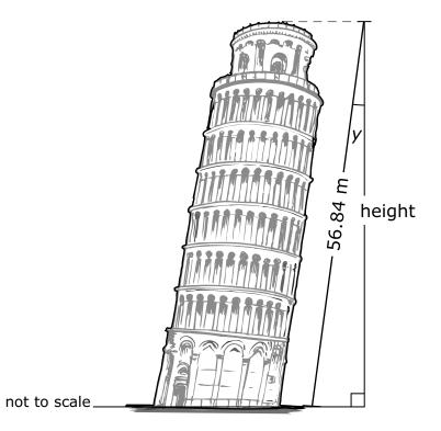
In the 1990s, engineers restored the building so that angle y changed from 5.5° to 3.99°.
