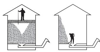
Figure 2. Bridged grain
