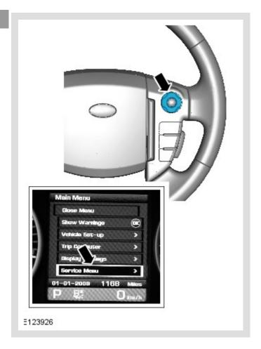
Press the right-hand directional button to access the instrument cluster menu.
