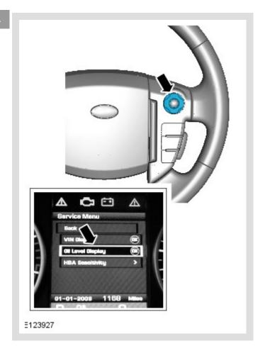
■ Press the right-hand directional button to access the Oil Level Display.
