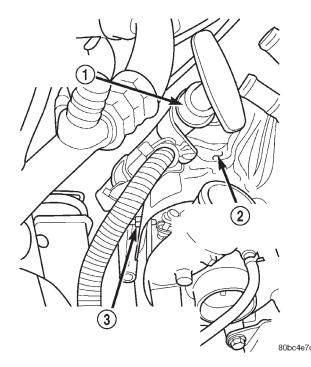
Fig. 23 Transmission Dipstick Tube Support Bracket
