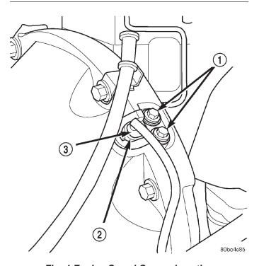
Fig. 4 Engine Speed Sensor Location
