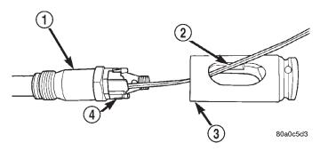
Fig. 38 Wiring Harness Through Socket
