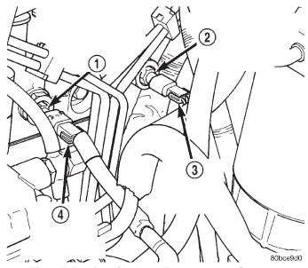
Fig. 25 Engine Coolant Temperature Sensors
