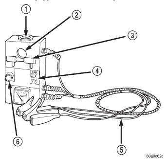
Fig. 12 Typical Glow Plug Tester
