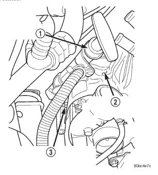
Fig. 20 Transmission Dipstick Tube Support Bracket
