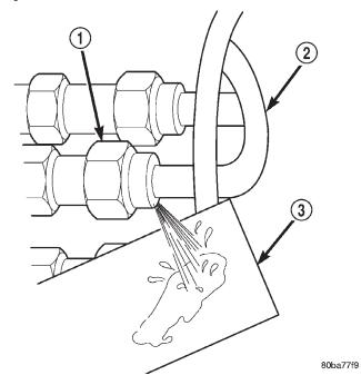
Fig. 17 Typical Fuel Pressure Test at Injection Pump
