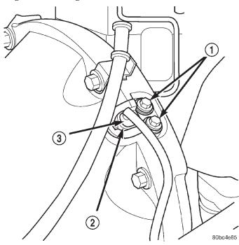
Fig. 17 Engine Speed Sensor Position & Orientation
