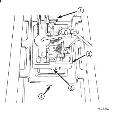
Fig. 23 Fuel Level Sensor Release Tab
