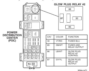
Fig. 14 Glow Plug Relay #2 Location
