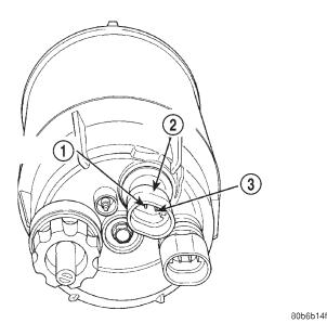
Fig. 8 Fuel Heater Temperature Sensor and Element Location
