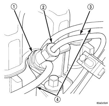
Fig. 39 Fuel Lines at Fuel Injectors
