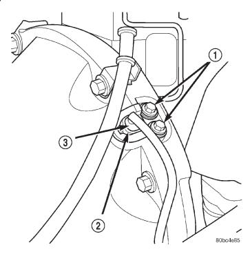
Fig. 21 Engine Speed Sensor
