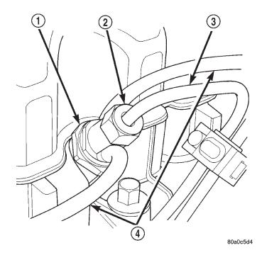
Fig. 19 Bleeding High-Pressure Fuel Line—Typical
