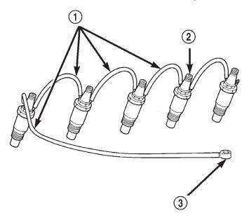
Fig. 7 Fuel Drain Tubes
