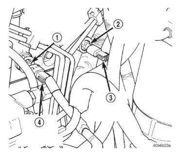
Fig. 26 Engine Coolant Temperature Sensors
