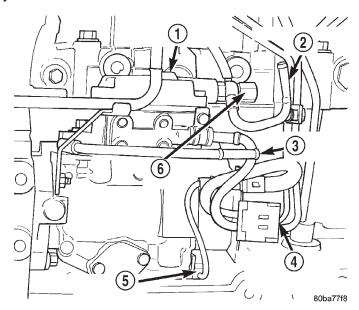
Fig. 7 Timing Solenoid
