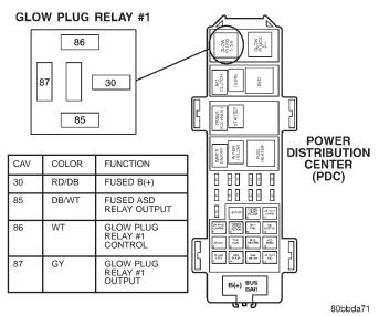
Fig. 8 Glow Plug Relay #1 Location
