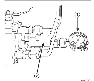
Fig. 34 Installing Dial Indicator and Special Adapter
