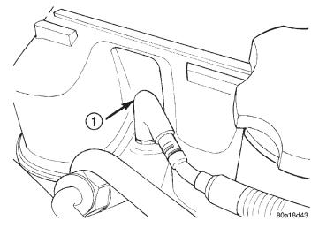
Fig. 15 Wiring Connection at Glow Plug
