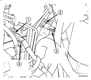
Fig. 11 Engine Coolant Temperature Sensor Location
