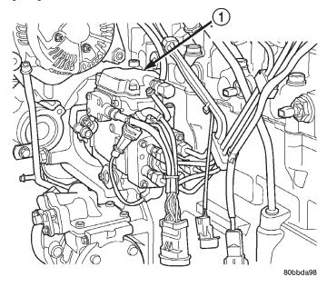
Fig. 3 Fuel Injection Pump
