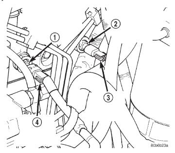
Fig. 3 Engine Coolant Temperature Sensor Location
