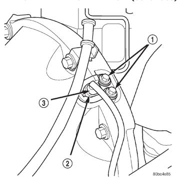
Fig. 22 Engine Speed Sensor
