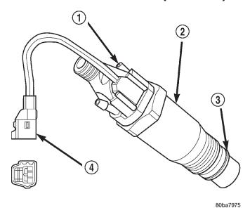
Fig. 16 Needle Movement Sensor Location
