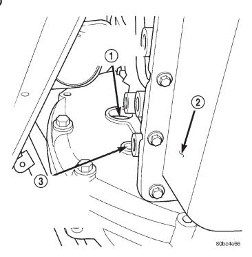
Fig. 35 Top Dead Center Alignment Tool Access Hole
