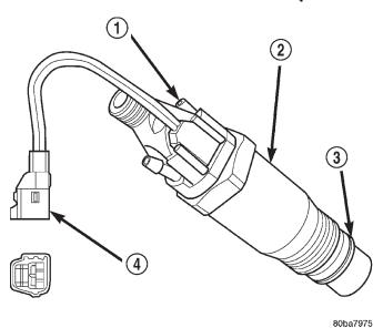
Fig. 2 Fuel Injector Sensor
