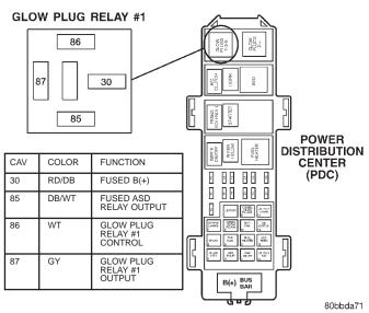
Fig. 13 Glow Plug Relay #1 Location
