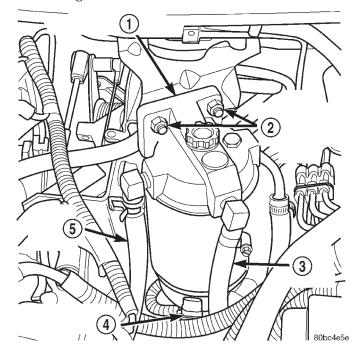
Fig. 2 Fuel Filter/Water Separator Location
