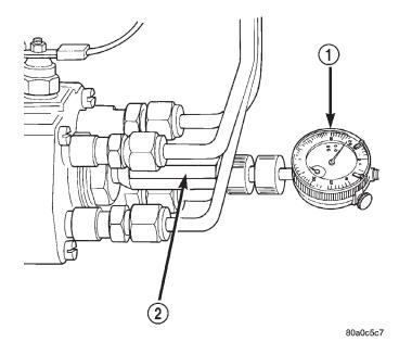
Fig. 28 Installing Dial Indicator and Special Adapter
