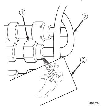
Fig. 1 Typical Fuel Pressure Test at Injection Pump
