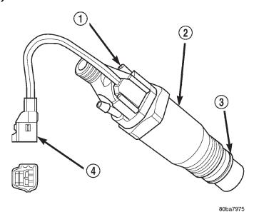
Fig. 5 Fuel Injector Sensor
