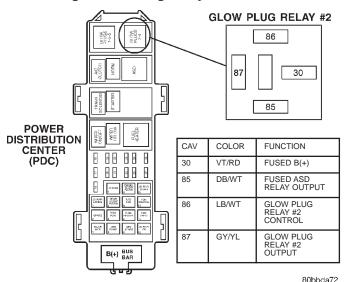
Fig. 9 Glow Plug Relay #2 Location
