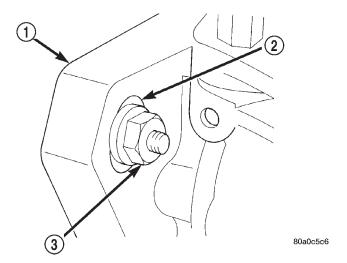
Fig. 32 Injection Pump Mounting Nuts
