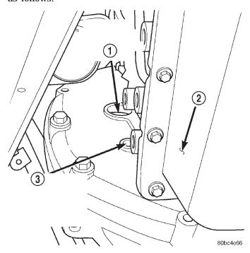
Fig. 26 Top Dead Center Alignment Tool Access Hole
