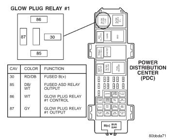
Fig. 10 Glow Plug Relay #1 Location
