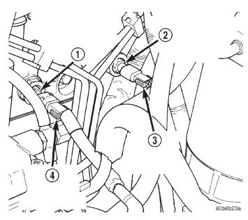
Fig. 13 Engine Coolant Temperature Sensor Locations
