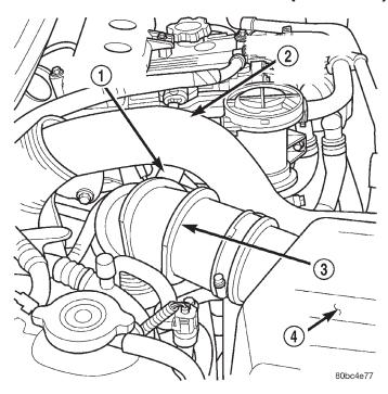
Fig. 25 Air Intake Hoses
