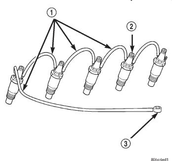
Fig. 20 Fuel Injectors and Drain Tubes
