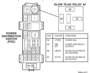
Fig. 11 Glow Plug Relay #2 Location
