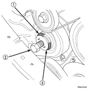
Fig. 31 Installing Pump Drive Gear Removal Tools
