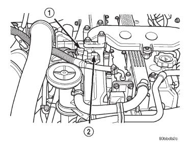
Fig. 16 Boost Pressure Sensor Location
