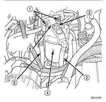
Fig. 21 Fuel Filter / Water Separator Position & Orientation
