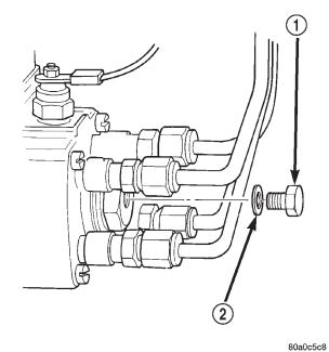
Fig. 33 Access Plug at Rear of Pump
