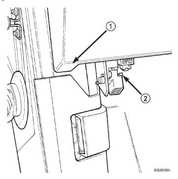
Fig. 5 Data Link Connector Location – L. H. D.
