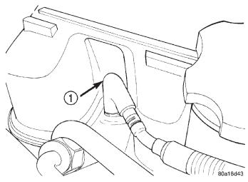
Fig. 28 Glow Plug Electrical Connector
