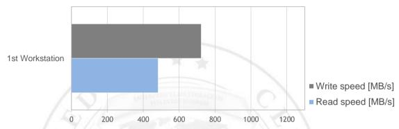
FIGURE 7: Single NIC performance test results chart for FUJITSU PRIMERGY 10Gb Network Controller (D2755)
