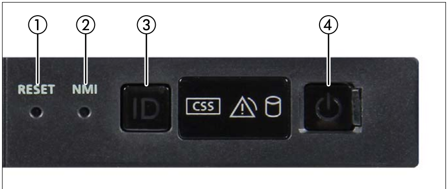
Figure 7: Controls on the front panel module
