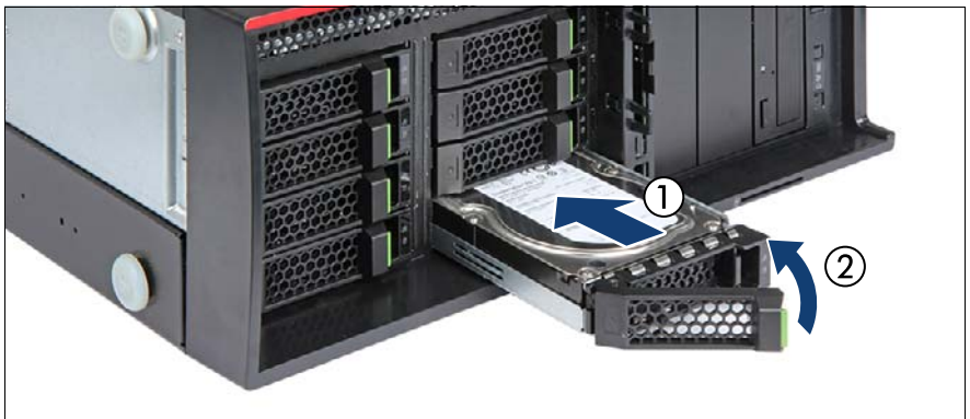
Figure 22: Installing the 3.5-inch HDD module
