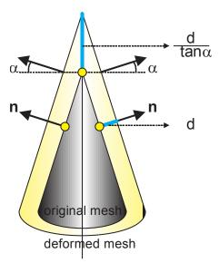
Figure 32: Local mesh shrinkage and/or expansion according to Eq. (4.1). Drawing from Ref [17]
