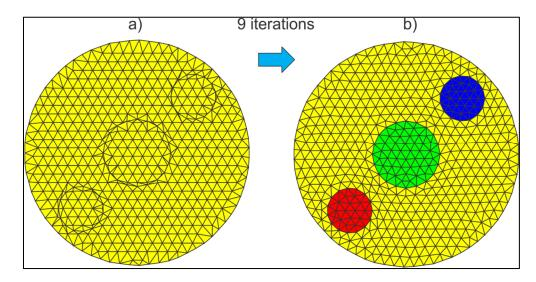
Figure 29: Results of Laplacian smoothing with algorithm *WCC* after 9<sup>th</sup> iteration. Drawing from Ref. [1]
