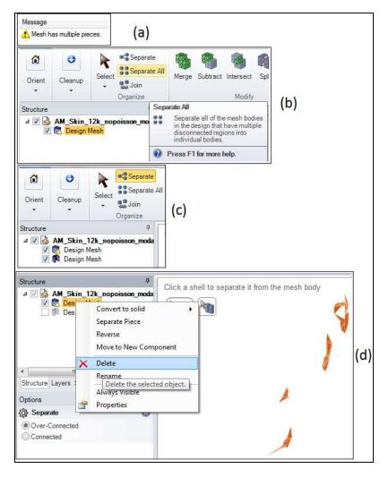
Figure 51: Resolving Multiple Pieces. Original Drawing in SpaceClaim
