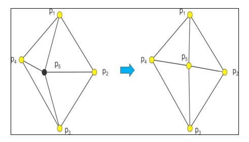
Figure 28: Concept of Laplacian smoothing. Drawing from Ref. [1]
