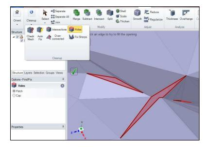
Figure 41: Non-Manifold Triangles Removed. Original Drawing in SpaceClaim
