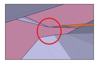
Figure 40: Non-Manifold Triangles Identified. Original Drawing in SpaceClaim
