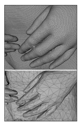
Figure 15: Original Mesh and Decimated Mesh. Original drawing
