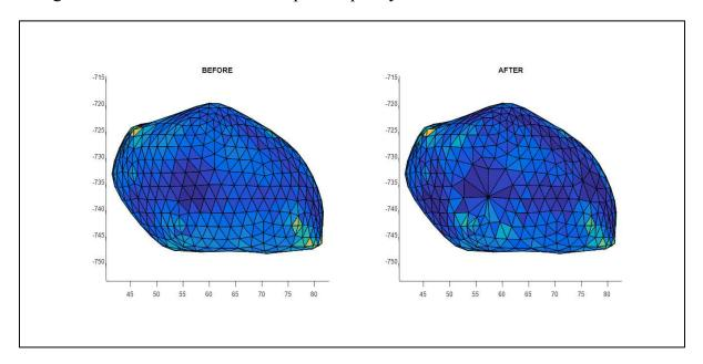
Figure 30: Decimation of Lower Curvature Area (25 iterations) with Local Laplacian Smoothing on Attached Nodes of Deleted Vertex. Original Drawing
