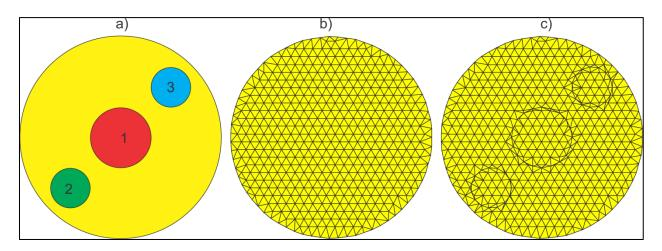
Figure 27: Problem geometry with non-intersecting boundaries and the initial meshes. Drawing from Ref.[1]
