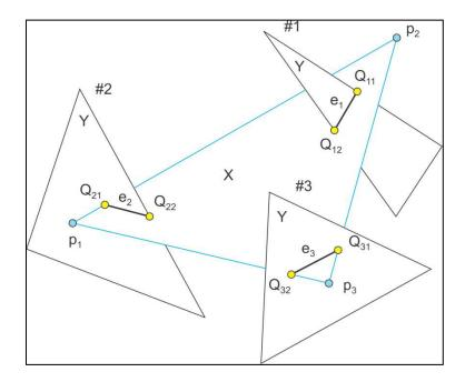
Figure 19: Three types of intersection of a triangle from a master mesh X with various triangles of a slave mesh Y. Cases #1 and #3 are equivalent if we treat the master and slave meshes as one set of triangles. Original Drawing from R.[10]
