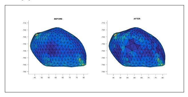
Figure 31: Decimation of Lower Curvature Area (25 iterations) with Local Laplacian Smoothing on More Nodes. Original Drawing
