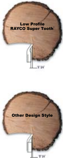
Tool Profile Comparison By comparing distance "A" to "B", you can see how the RAYCO Super Tooth® increases the strike point clearance and eliminates tool drag on the stump.
