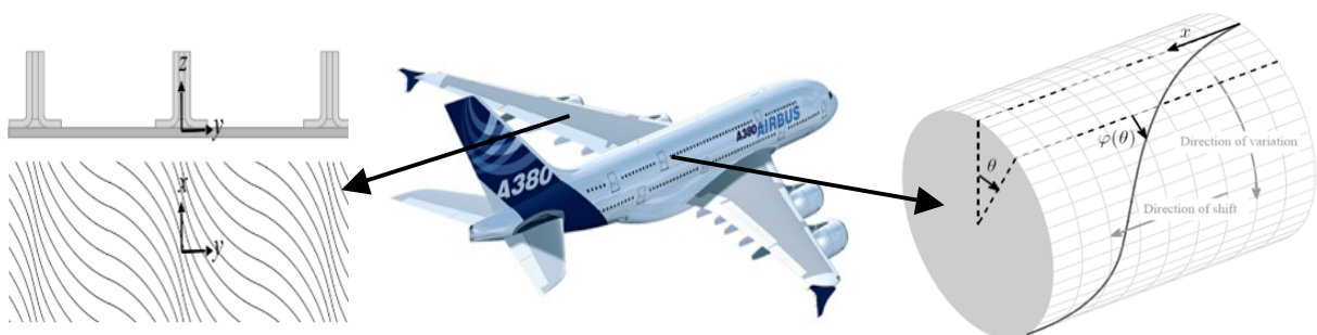
Figure 1. Examples of fibre steered designs of a wing skin and a fuselage section [2]
