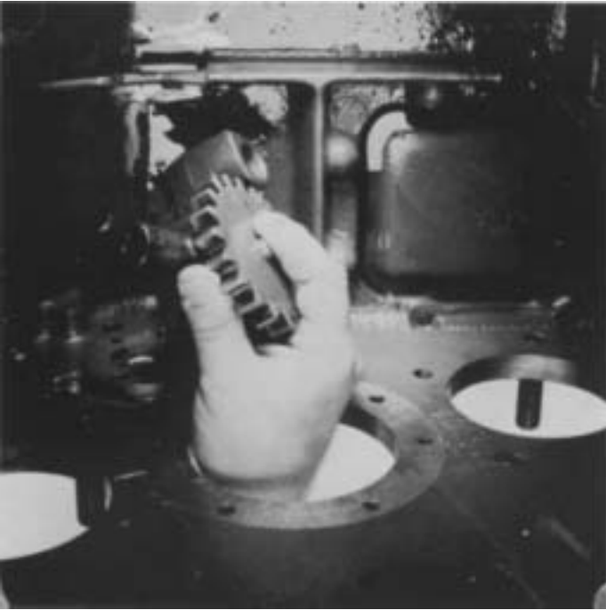
3. Remove the integral oil pump from case.
