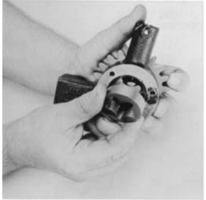
5. Remove outer oil pump element from pump.
