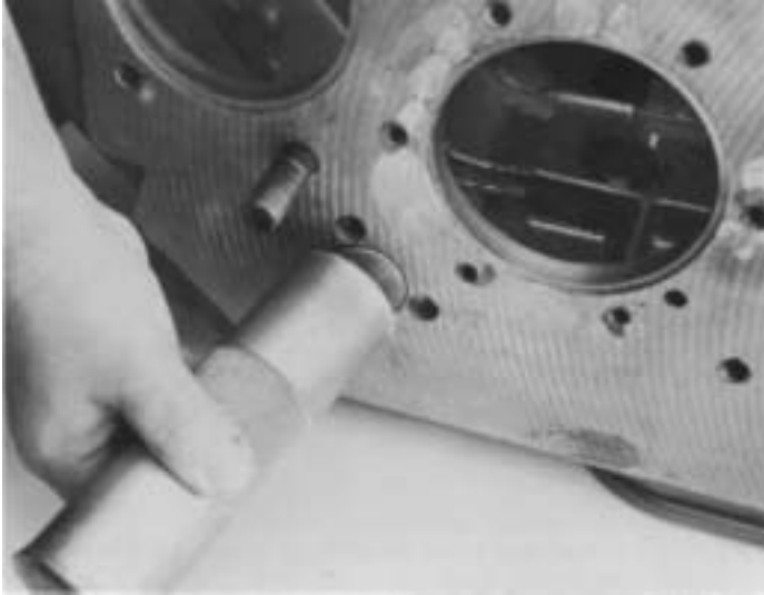
1. Replace O-ring on front case plug. Seat plug in front case bore with a maul.
