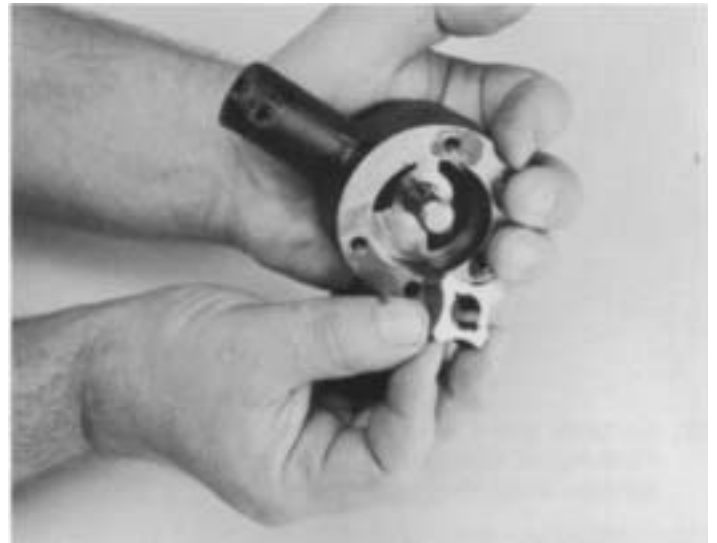
10. Remove internal oil pump element from drive shaft.
