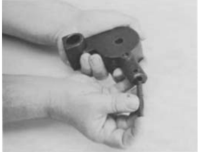
3. Install relief valve spring in oil pump housing.
