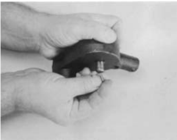
8. Remove key from drive shaft keyway.
