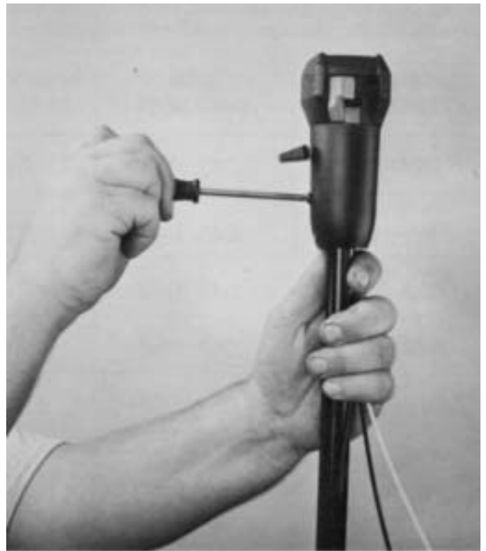
11. Position valve cover on Roadranger valve and secure by tightening the two mounting screws in cover,
