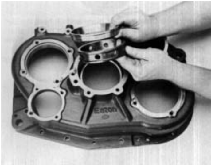
8. Install rear bearing race and rear bearing outer spacer in auxiliary housing bearing bore. The bearing race will be at proper depth when race shoulder is seated on top of bearing bore.
