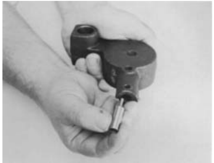
14. Remove relief valve from housing bore.
