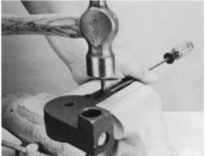
4. Secure oil pump housing in a vice. Depress spring in housing bore and drive relief valve retention roll pin into roll pin bore.
