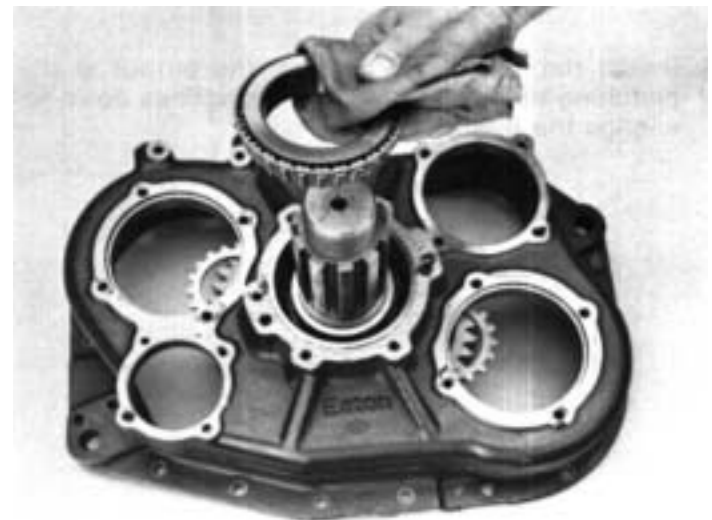
10. Heat the rear bearing cone and install on the shaft, taper side down and inside the cup. Make sure the lip of the rear bearing cup is fully seated on the housing with the bearing installed.
