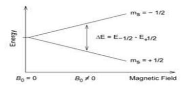
Fig 2: Relationship between energy and magnetic field
