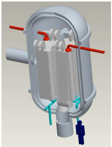
**Fig. 2** Baseline 50 MW(t) IHX design. Hot, high-pressure helium enters from the bottom and exits from the side of the IHX pressure vessel.
