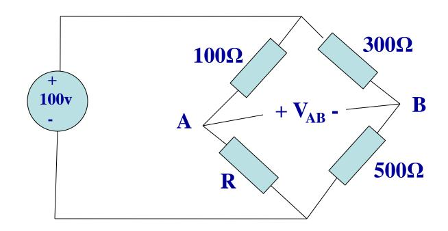
•  $V_{BD} = 100 \text{ v} \cdot 500\Omega/(300+500)\Omega = 62.5 \text{ v}$
