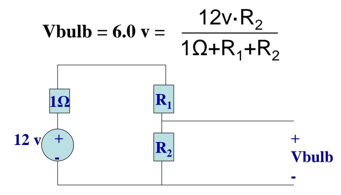
• The parallel combination of ten  $100\Omega$ bulbs is  $10\Omega$ , the parallel combination with R2 is  $\frac{10 \cdot R_2/(10+R_2)}{10 \cdot R_2/(10+R_2)} \Omega$
