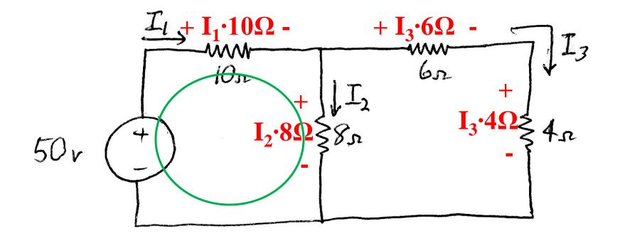
Write 1<sup>st</sup> Kirchoff's voltage law equation -50 v +  $I_1$ ·10 $\Omega$  +  $I_2$ ·8 $\Omega$  = 0
