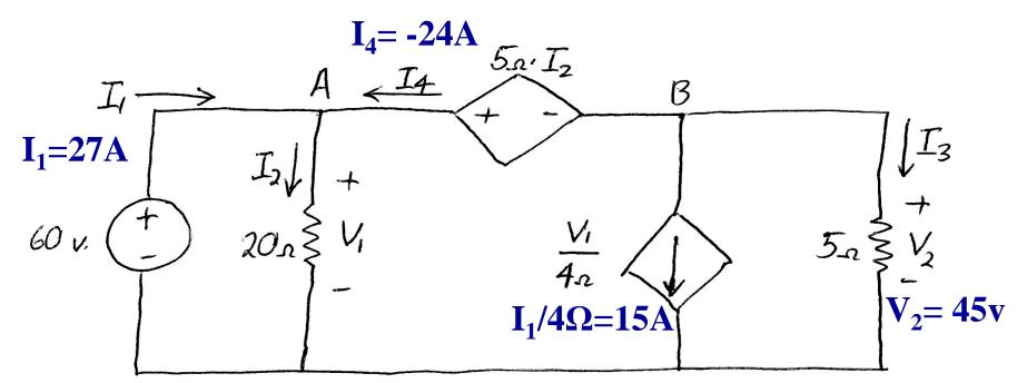
60 v source generating, P=-27A-60v=-1620 watts 5-I<sub>2</sub> source absorbing, P=24A-15v=360 watts V<sub>1</sub>/4 source absorbing, P=15A-45v= 675watts
