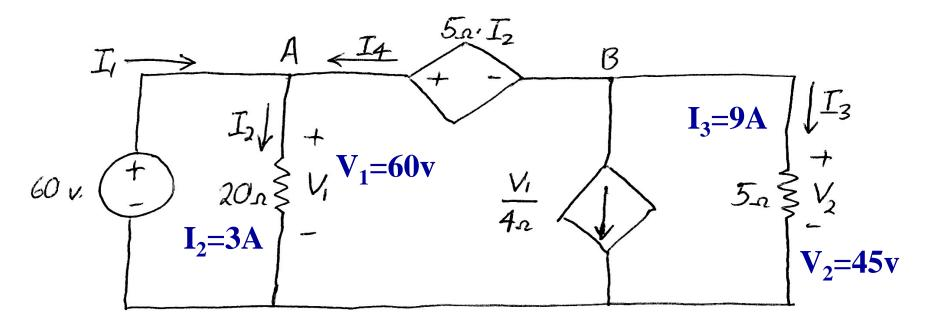
20  $\Omega$  resistor absorbing, P=3A-60v=180 watts 5  $\Omega$  resistor absorbing, P=9A-45v= 405 watts -1620 w +360 w + 675 w + 180 w + 405 w = 0
