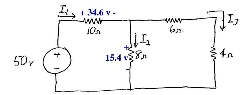
If  $I_2 \cdot 8 \Omega = 15.4 \text{ v}$ , then  $I_2 = 15.4/8 = 1.93 \text{ A}$ By KCL,  $I_1 \cdot I_2 \cdot I_3 = 0$ , so  $I_3 = I_1 - I_2 = 1.53 \text{ A}$
