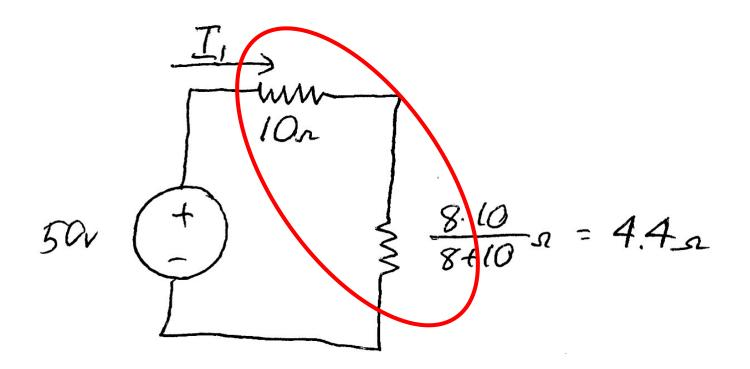
The 10 and 4.4 ohm resistors are in series, so are combined into  $10+4 = 14.4\Omega$
