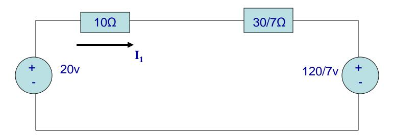
• Rtotal=100/7  $\Omega$  and Vtotal=20/7 volts
