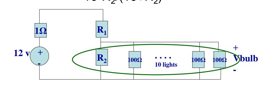
Using the voltage divider and the minimum voltage allowed:
