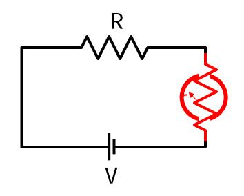
Any ammeter has a resistance r. The current you measure is
