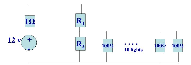
The voltage across each bulb must be within the range of 5.5 to 6 volts in order for the bulbs to be bright enough. Find R<sub>1</sub> and R<sub>2</sub>.
