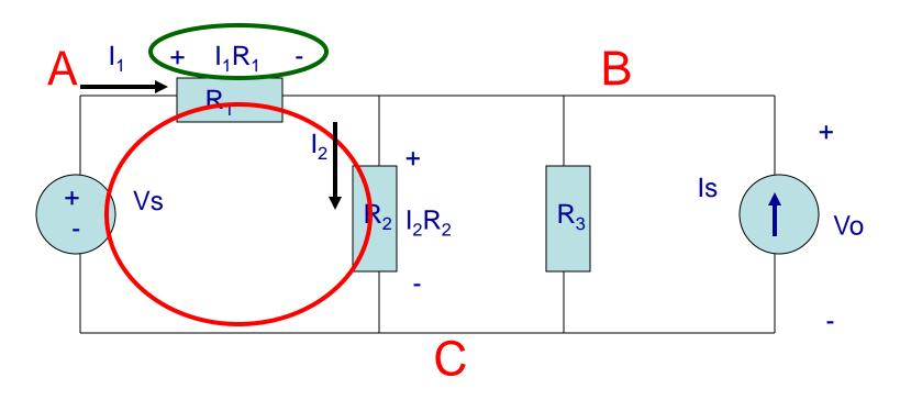
Starting at node A, add the  $1^{st}$  voltage drop: +  $I_1R_1$
