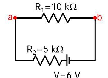
$$V_{ab} = IR = (0.4 \times 10^{-3})(10 \times 10^{3} \Omega) = 4 V$$
