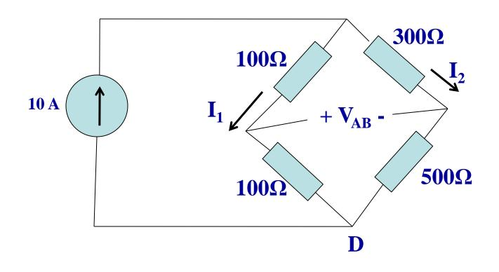
• First, simplify by combining the series resistances in each branch of the bridge
