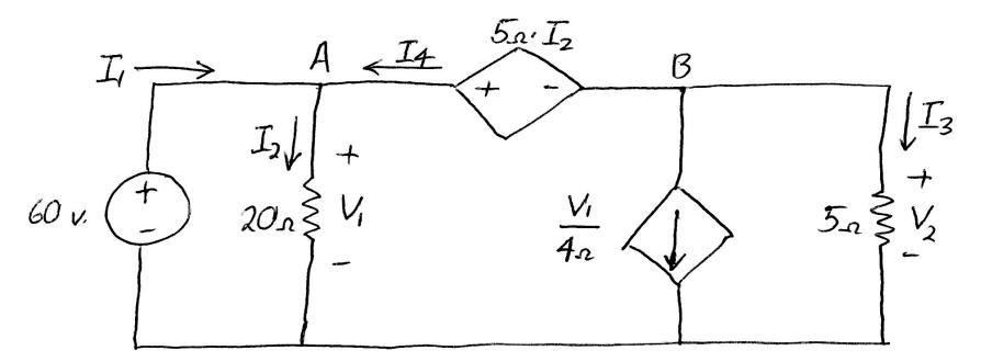
Writing Kirchoff's Current law at B  $I_4 + I_3 + V_1/4 = 0$  (all leaving node B) Since  $V_1/4\Omega = 15$  A and  $I_3 = 9$  A,  $I_4 = -24$  A
