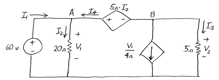
Writing Kirchoff's Voltage law around the outside loop, -60 v +  $5\Omega \cdot I_2 + 5\Omega \cdot I_3 = 0$  where  $I_2=3$  A, so  $I_3 = (60-15)v / 5\Omega = 9$  A
