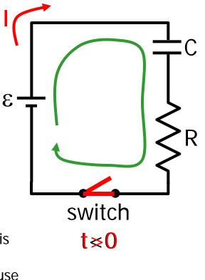
\*Convention for capacitors is "like" batteries: negative if going across from + to -.
