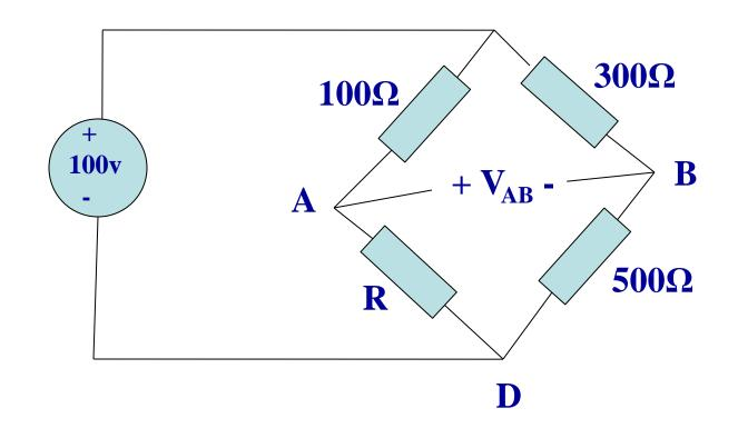
• The Wheatstone bridge is considered balanced when  $V_{AB}=0 v$ .
