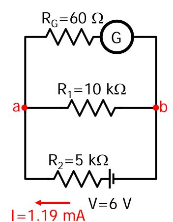
To reduce the percent error, the device being used as a voltmeter must have a very large resistance, so a voltmeter can be made from galvanometer in series with a large resistance.
