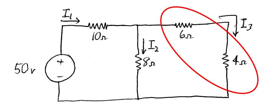
The 6 and 4 ohm resistors are in series, so are combined into  $6+4 = 10\Omega$
