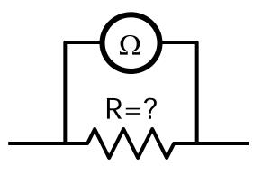
To measure a really small resistance, an ohmmeter won't work.
