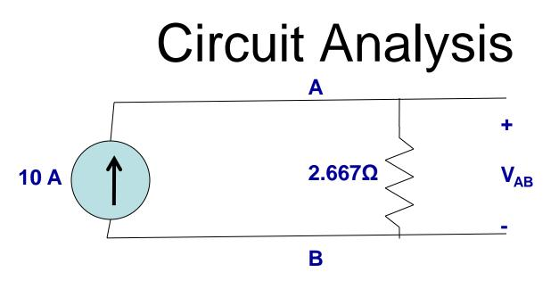
By Ohm's Law:  $V_{AB} = 10 \text{ A} \cdot 2.667 \Omega$ So  $V_{AB} = 26.67$  volts
