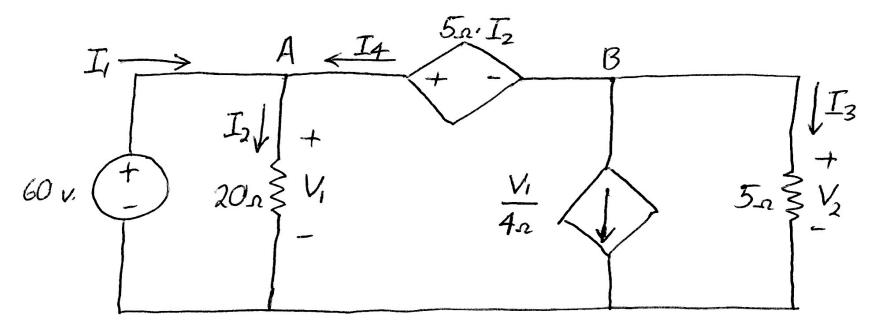
If  $I_2 = 3$  A, then the 5 $\Omega \cdot I_2$  dependent source is 15 volts and if  $V_1 = 60$  v., then the  $V_1/4\Omega$ dependent source is 15 A
