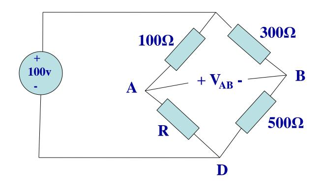
• Find the Voltage at B, using the voltage divider theorem
