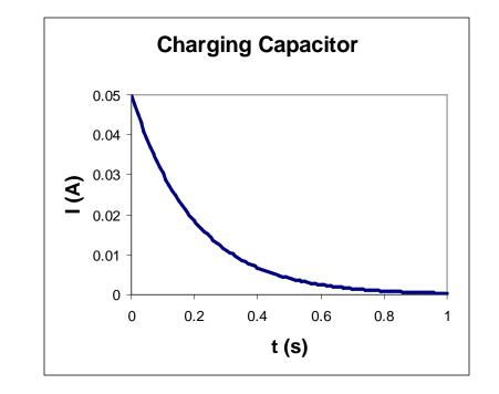
Sample plots with  $\epsilon{=}10$  V, R=200  $\Omega,$  and C=1000  $\mu\text{F}.$  RC=0.2 s
