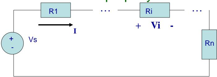
• You can design a voltage divider circuit to produce the necessary voltages
