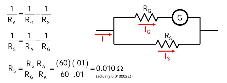
The shunt resistance is chosen so that  $I_G$  does not exceed the maximum current for the galvanometer and so that the effective resistance of the ammeter is very small.
