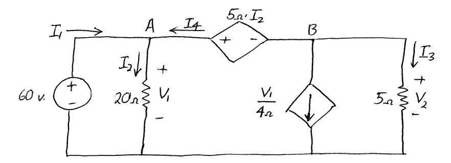
$V_1 = 60$  volts because the 20Ω resistor is in parallel; by Ohm's law,  $V_1 = I_2 \cdot 20\Omega$ ; so  $I_2 = V_1/20\Omega = 60v/20\Omega = 3$  A
