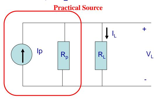
V<sub>L</sub> and I<sub>L</sub> must be the same in both circuits for R<sub>L</sub>= 0, or a short circuit
