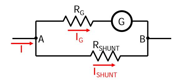
Homework hint: "the galvanometer reads 1A full scale" means a current of  $I_G$ =1A produces a full-scale deflection of the galvanometer needle. The needle deflection is proportional to the current  $I_G$ .
