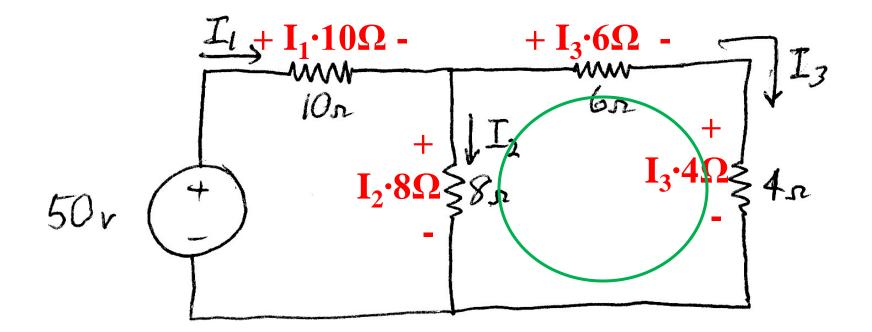
Write 2<sup>nd</sup> Kirchoff's voltage law equation  $-I_2 \cdot 8\Omega + I_3 \cdot 6\Omega + I_3 \cdot 4\Omega = 0$ or  $I_2 = I_3 \cdot (6+4)/8 = 1.25 \cdot I_3$
