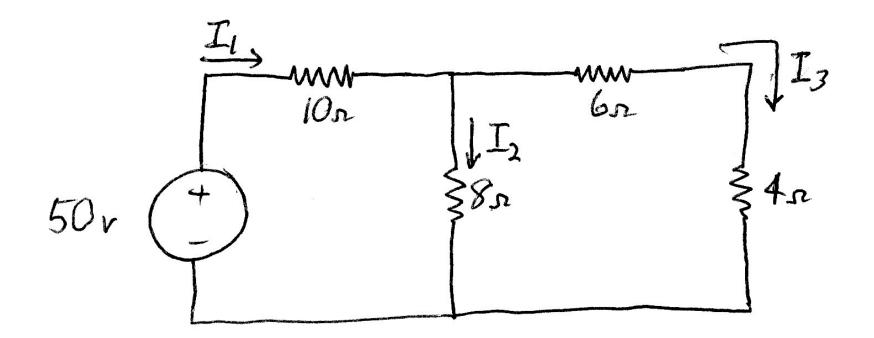
Solve for the currents through each resistor And the voltages across each resistor
