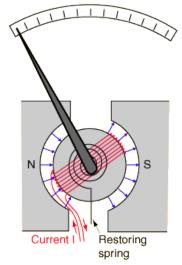
A typical galvanometer has a resistance of a few tens of ohms.
