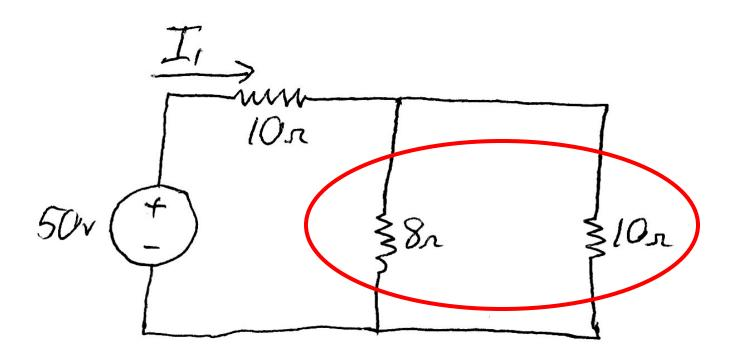
The 8 and 10 ohm resistors are in parallel, so are combined into  $8\cdot10/(8+10) = 14.4 \Omega$
