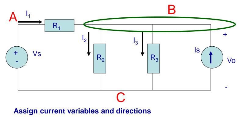
Add currents in, subtract currents out:  $I_1 - I_2 - I_3 + I_3 = 0$
