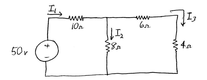
Solve for the currents through each resistor And the voltages across each resistor using Series and parallel simplification.
