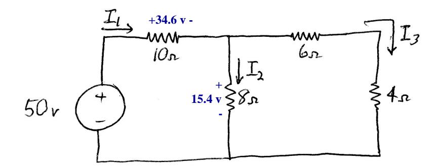
If  $I_1 = 3.46$  A, then  $I_1 \cdot 10 \ \Omega = 34.6$  v So the voltage across the 8  $\Omega = 15.4$  v
