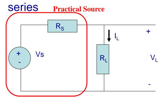
We want to create an equivalent using a current source and parallel resistance for any R<sub>L</sub>
