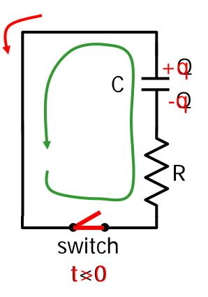
\*Convention for capacitors is "like" batteries: positive if going across from - to +.
