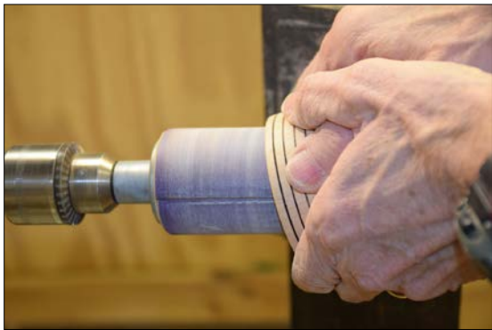
Photo 8: Sanding the parted edge using a sanding cylinder on the lathe.
