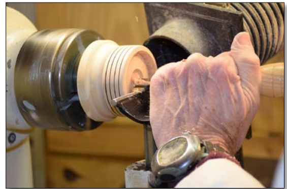
Photo 5: Hollowing the inside of the bracelet using a spindle gouge cutting outward toward the rim.
