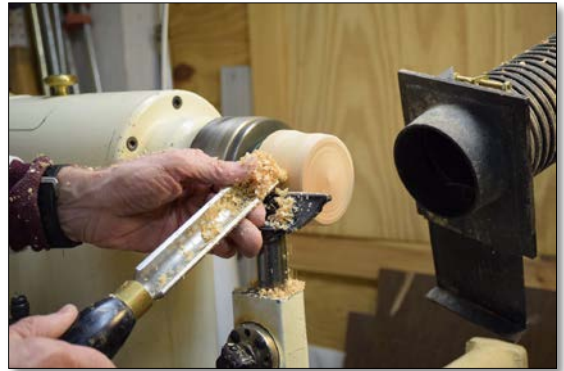
Photo 1: Using a roughing gouge to turn a piece of maple to a cylinder 3 inches in diameter and about 2 inches long.
