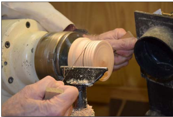
Photo 3: Using a wire to burn boundary markings.
