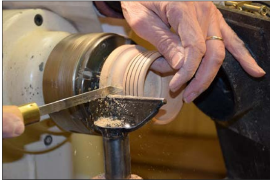
Photo 7: Parting off the bracelet with a skew and preparing to catch the bracelet with one finger inside the bracelet.
