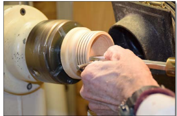
Photo 6: Using a straight edge scaper parallel to the ways of the lathe to make the inside of the bracelet parallel to the outside of the bracelet.
