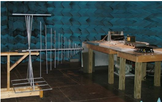
Radiated Emissions Test Setup
