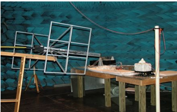
Radiated Immunity Test Setup
