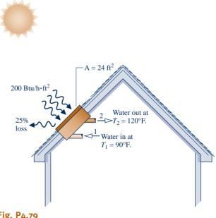
energy from the sun at a rate of 200 Btu/h per ft<sup>2</sup> of collector surface. Twenty-five percent of the incoming energy is lost to the surroundings. The remaining energy is used to heat domestic hot water from 90 to 120°F. The water passes through the solar collector with a negligible pressure drop. Neglecting kinetic and potential effects, determine at steady state how many gallons of water at 120°F the collector generates per hour.
