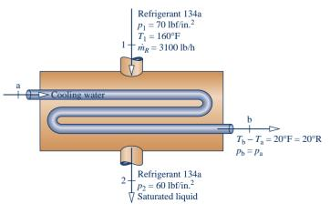
cooling water increases in temperature by 20°F and experiences no significant pressure drop. Cooling water can be modeled as incompressible with v = 0.0161 ft<sup>3</sup>/lb and c = 1 Btu/lb · °R. The mass flow rate of the refrigerant is 3100 lb/h. Neglecting kinetic and potential energy effects and ignoring heat transfer from the outside of the condenser, determine
