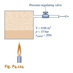
the pressure constant in the tank by allowing saturated vapor to escape. Neglecting kinetic and potential energy effects
