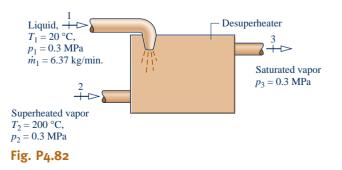
determine the mass flow rate of the incoming superheated vapor, in kg/min.
