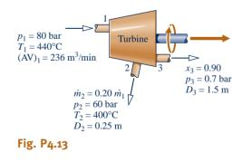
exits through a diameter of 1.5 m with a pressure of 0.7 bar and a quality of 90%. Determine the velocity at each exit duct, in m/s.
