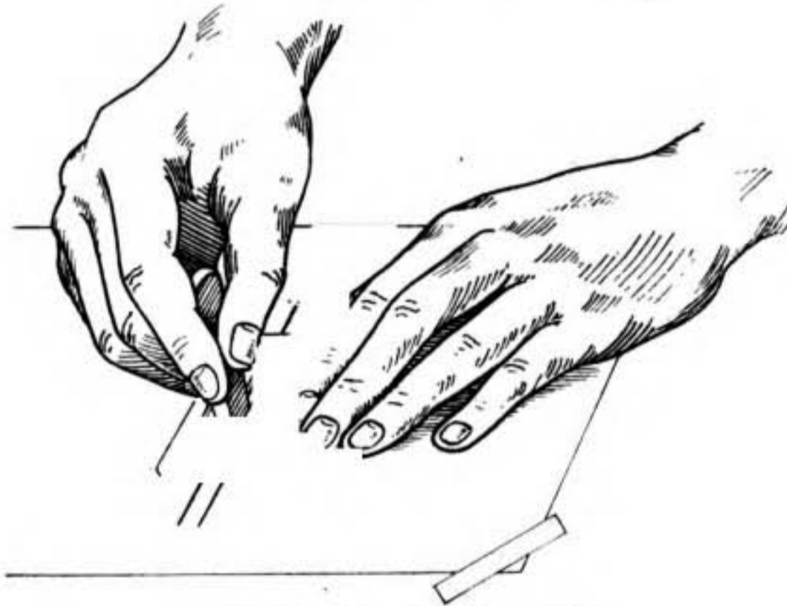
FIGURE 4.—Use of erasing shield.
