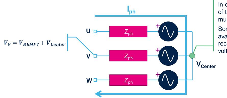
In order to detect the zero-crossing of the BEMF the center-tap voltage must be known.
