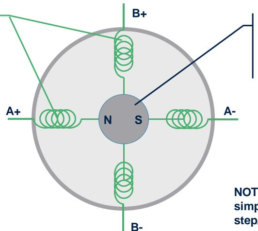
A permanent magnet generates the magnetic field of the rotor
