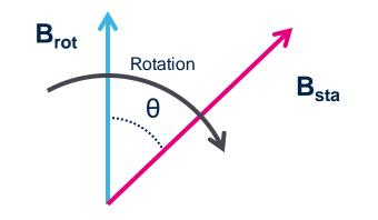
$Tq \propto B_{rot} \cdot B_{sta} \cdot \sin(\theta) \propto I_{ph} \cdot \sin(\theta)$
