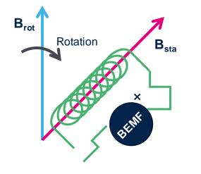
Consequently an electro-motive force facing the flux variation is generated (Lenz's law). This effect is named **back electro-motive force** (aka **BEMF**) and it is proportional to the motor speed according to the formula:
