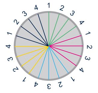
Example: in a 20 steps stepper motor each full step combination (numbered from 1 to 4) can position the rotor at 5 possible angles (colors)
