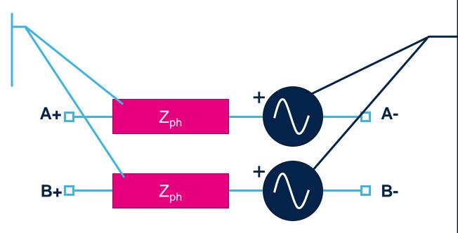
Back electromotive force generator. BEMF are two sinewave voltages<sup>(\*)</sup> delayed from each other by 90°. The sinewave amplitude is proportional to the motor speed:
