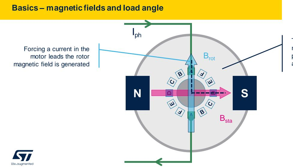
The torque applied to the rotor is the highest possible because the load angle ( $\theta$ ) is about 90°
