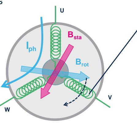
When the magnetic field of the rotor crosses the unloaded phase, the respective BEMF voltage changes polarity (zerocrossing)
