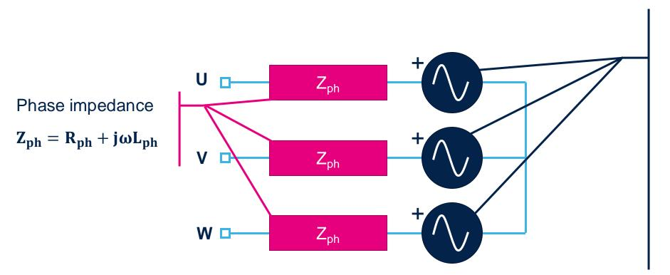
Back electromotive force generators. BEMFs are three sinewave voltages<sup>(\*)</sup> delayed from each other by 120°.
