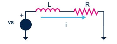
Scenario 1 (ON time) Inductance is charged applying a voltage:
