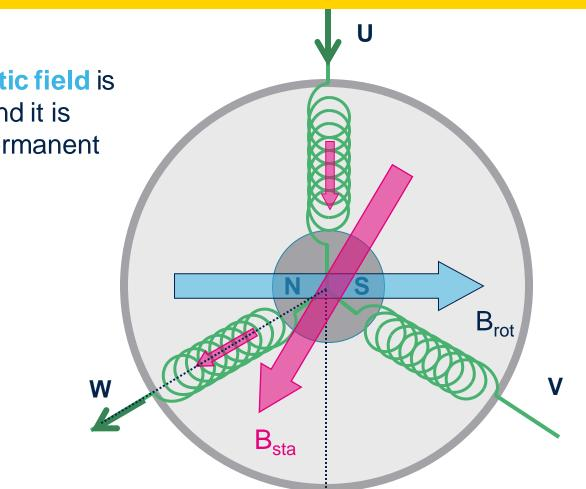
When a current flows from a motor phase to another one the magnetic fields are combined generating the stator field.
