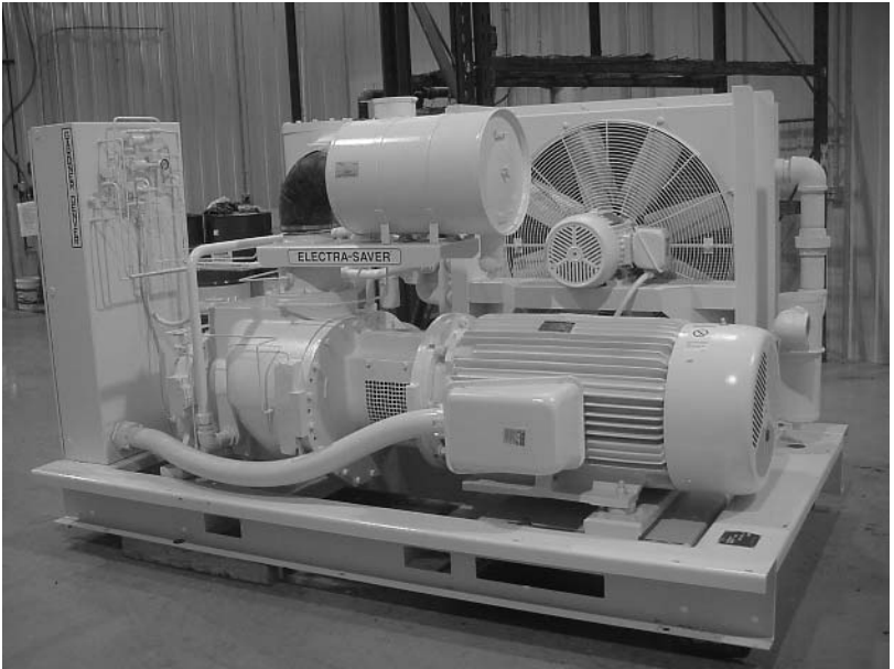
Figure 4-5. Include the 100 HP motor with the compressor.
