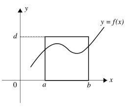
Figure 13.1 Area under f to be calculated, using the Monte Carlo method.
