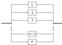
Figure 9.2 Geometric representation for a parallel system.
