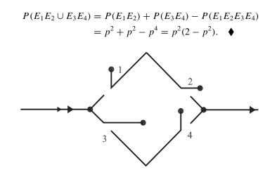
Figure 3.8 Electric circuit of Example 3.32.
