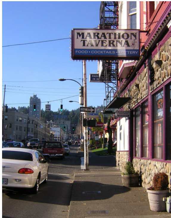
Figure 1. Traffic controls such as official signs need to be close to the road, distinctive from other information presentations, brief, and explicit. This photo provides an example of signs that are close to the road but may be confused with background information.
