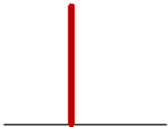
Frequency spectrum of a sine wave, periodic in the sample period T.
