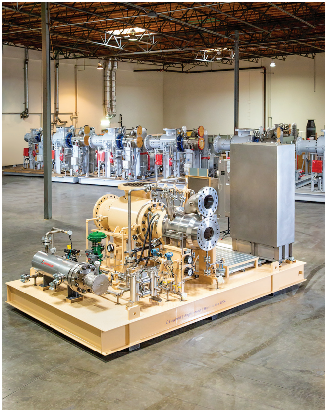
FIG. 4. Active magnetic bearing turboexpander-compressor with on-skid controller. Photo courtesy of L.A. Turbine.
