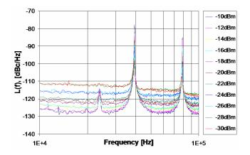
Figure 9. PM noise measurement of the spurious levels and far-fromcarrier noise as master-to-slave injection is varied.
