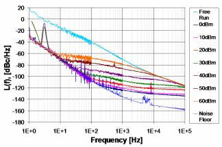
Figure 4. PM noise measurement of the slave OEO injection locked to a SLCO at various injection levels at 10 GHz. Top plot has no injection; bottom plot is the SLCO-only PM noise. Note: injection powers represent negative dBm.
