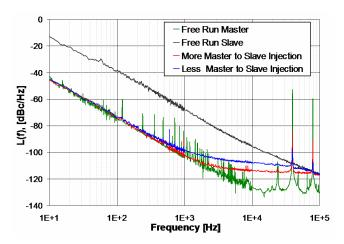
Figure 8. Dual injection-locked OEO with fixed slave-to-master injection at 9.953 GHz. Note the far-from-carrier noise floor increase with less master-to-slave injection, while the spurious levels decrease.
