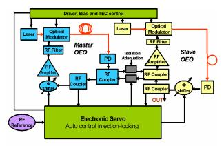
Auto Control of the Injection-locked Dual OEO
