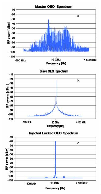
Figure 2. RF Spectrum of (a) Master OEO, (b) Slave OEO and (c) Injection Locked OEO at 10 GHz.
