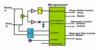
Figure 11. Proposed automatic control of the DIFO.
