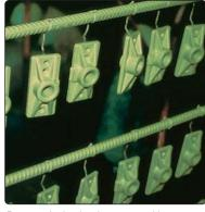
Post-tensioning hardware coated in accordance with AASHTO and ASTM specifications with 3M™ Scotchkote™ 413 spray grade.
