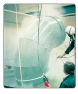
Fluid bed dip application of 3M<sup>™</sup> Scotchkote<sup>™</sup> 206N.
