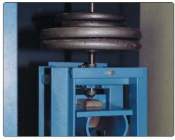
Gouge test simulates the stresses on a coating during a horizontal pipe pull. The coating sample is dragged under a weighted bit and the gouge depth is measured. Photo courtesy of Technical Inspection Services, Inc. (TISI). Houston, Texas
