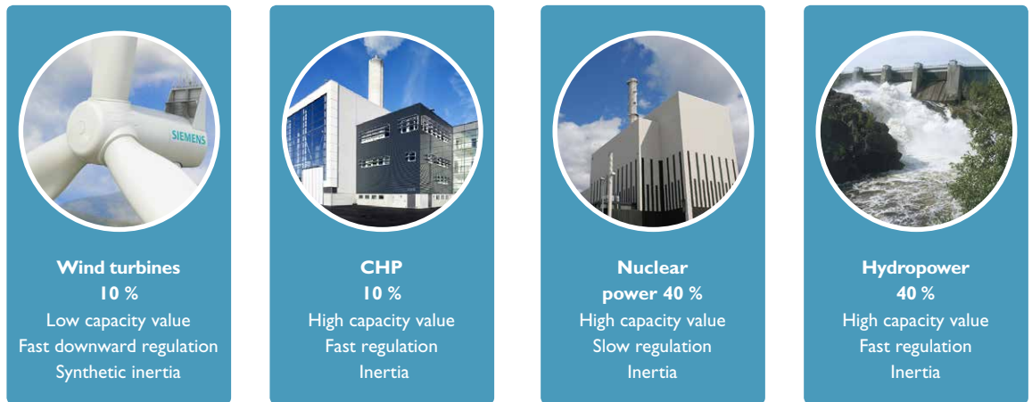
Figure 4: Summary of the energy sources' properties and their share of electricity production today. Source: Electricity Crossroads Production work group 2015.
