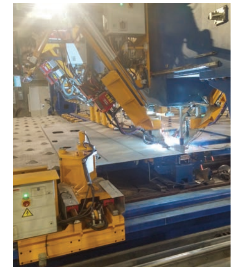
The operator of our single sided welding machine can complete the equivalent of 24 hours of manual welding in 20 minutes with a 99% accuracy rate
