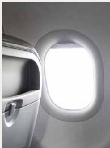
PLEXIGLAS® GS 249 stretched for passenger cabin windows.
