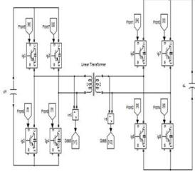
Fig3. Bi-directional DC-DC Converter
