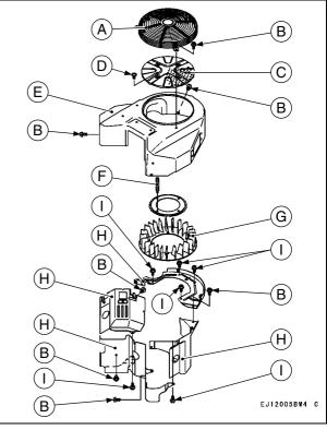
A. Guard B.D.F.I. Bolt C. Air Inlet Screen E. Fan Housing G. Cooling Fan H. Shroud
