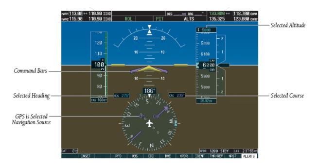
The above PFD view on the AFSC line displays default view of what you will see when the 'FD' button is pressed and the Flight Director System is active. The following roll modes will be annunciated when the appropriate button is selected:
