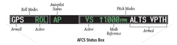
The only indication that the autopilot is engaged is seen in the above AFCS Status Box view.
