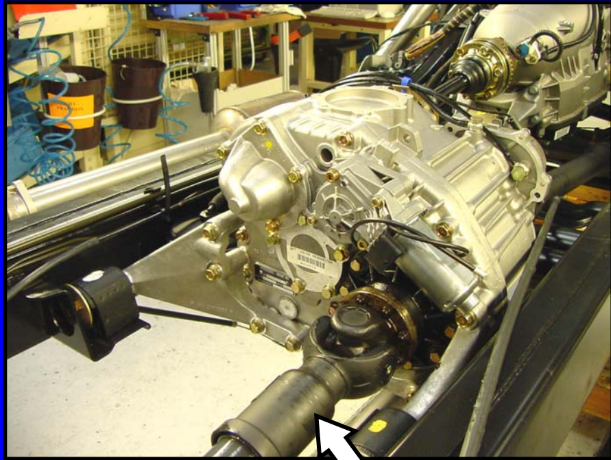
Propeller shaft to rear differential
