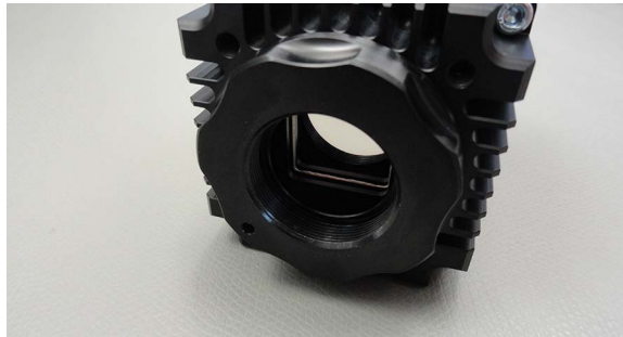
Figure 102: Camera mount without filter, directly exposing the sensor
