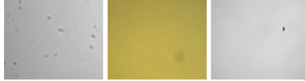
Figure 101: Examples for the appearance of dust on the filter (left and middle), and the sensor (right)
