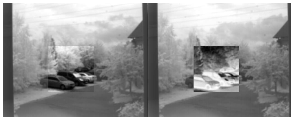
Figure 92: Left: Auto contrast applied to a ROI in the usual way, right: auto contrast with the ContrastAutoIntensity values reversed.
