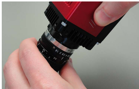
Figure 100: Illustration of camera orientation when removing lens or dust cap
