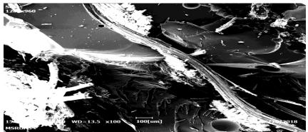
Fig. 11 shows tensile fracture of hybrid composites using hand layup techique
