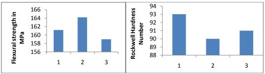
Fig. 8 shows the Flexural strength and Hardness of the composite material
