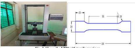
Fig. 3. Shows the UTM with tensile specimen
