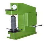
Fig.5. Shows the Rockwell hardness tester
