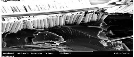
Fig. 12 shows tensile fracture of hybrid composites using vaccum bagging techique
