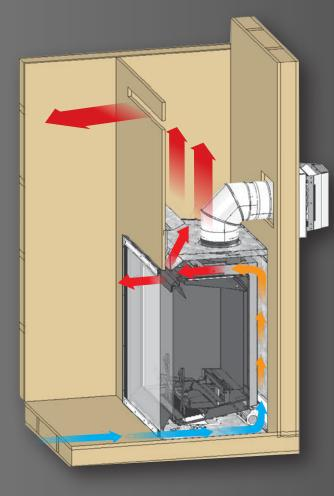
Convective heat that rises from the fireplace is captured in the chase and channeled through the vent using the Cool Surface System.
